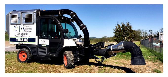
Blowing litter will always be a problem for the landfill. This unit will give us the ability to more easily pick up litter in all weather conditions. The life cycle for this unit is 8 years. We are recommending the purchase of this unit for \$132,960. The unit comes with a 2 year/2000-hour warranty and has a 4-month lead time.
